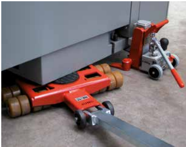
Castors with ball bearings guarantee easy movement.
