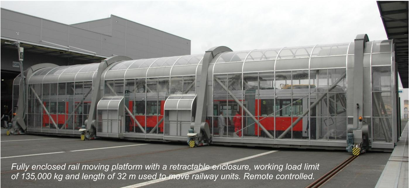
*Fully enclosed rail moving platform with a retractable enclosure, working load limit of 135,000 kg and length of 32 m used to move railway units. Remote controlled.*
