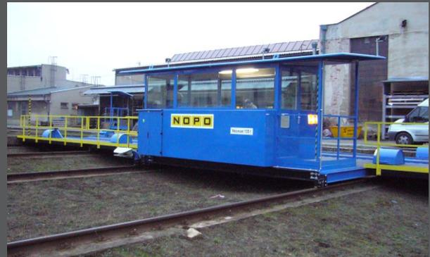
▲ Recessed rail moving platform with working load limit of 135,000 kg and a length of 24 m for the transport of railway units. Semi-automatic controls from the cab.
