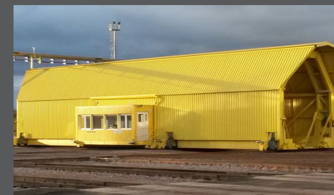
Above-grade fully enclosed rail moving platform with working load limit of 80,000 kg and a length of 30 m with wedge ramps for the transport of railway units.
