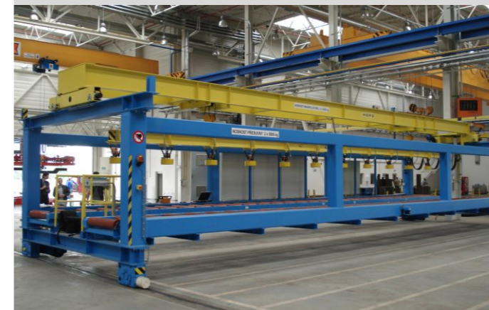
Above-grade fully enclosed rail moving platform with working load limit of 80,000 kg and a length of 30 m with wedge ramps for the transport of railway units.
