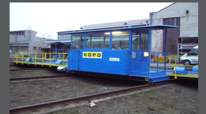
Recessed rail moving platform with working load limit of 135,000 kg and a length of 24 m for the transport of railway units. Semi-automatic controls from the cab.
