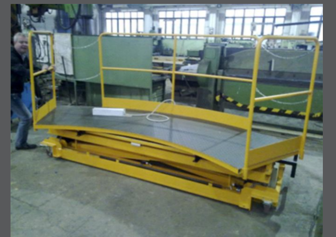
▲ Traverser on tires with special enclosure.
