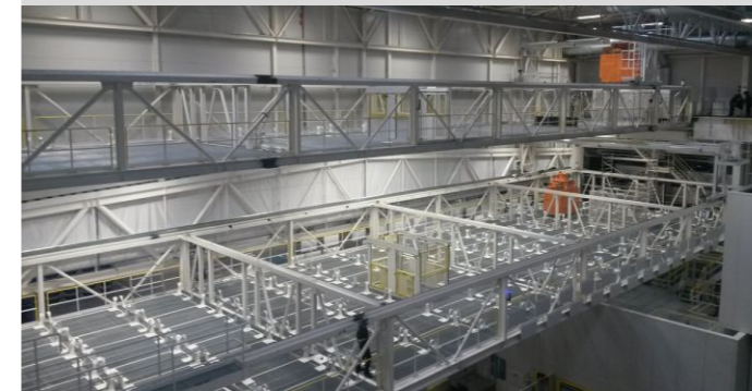
Telescopic manipulator with rotation and forks.
