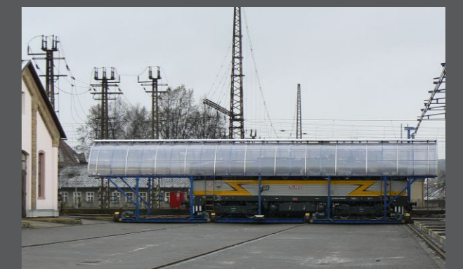
Recessed, partially enclosed rail moving platform with working load limit of 120,000 kg and length of 21 m for the transport of railway units. Semi-automatic controls from the cab.
