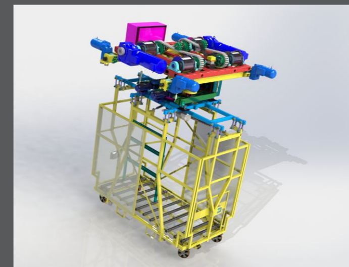
Telescopic manipulator with rotation and forks.
